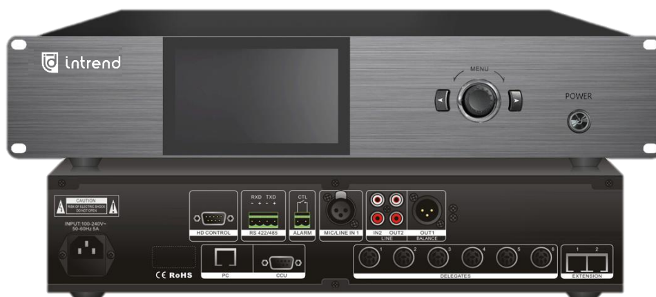
Figure 3.1 Digital Interpretation Host ICS-PRO-CU
